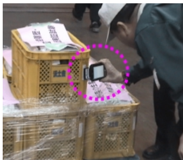
Fig. 8. Reading RFID tags which were pasted on container cases in the coop delivery center, using a mobile RFID-reading device.
