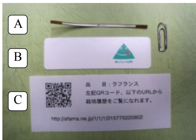
Fig. 4. RFID tags, and a barcode label which were used in the practical experiments.
