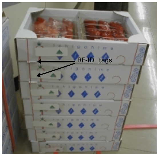
Fig. 5. RFID tags which are attached on to the cardboard boxes containing strawberry fruits at the wholesale market.
